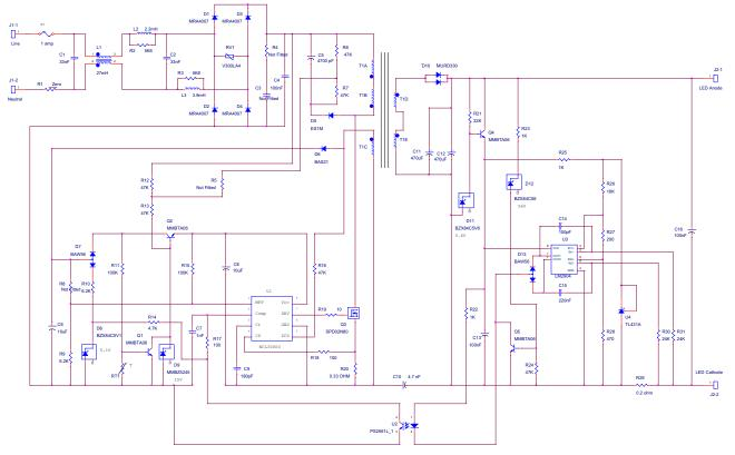
Figure 6. Schematic for 277 Vac optimized EMI filter
