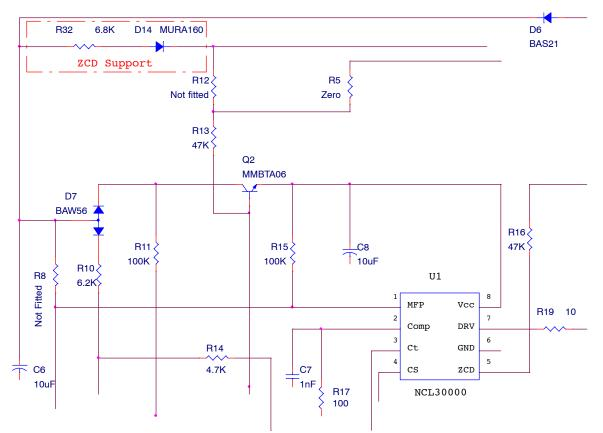
Figure 10. Partial Schematic Showing ZCD Support Circuit
