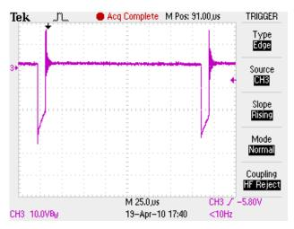
Figure 4. High Leakage Inductance with Minimum Off-Time
