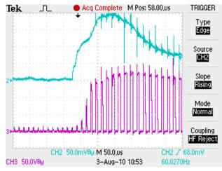
Figure 8. Switching waveforms after TRIAC turns on
