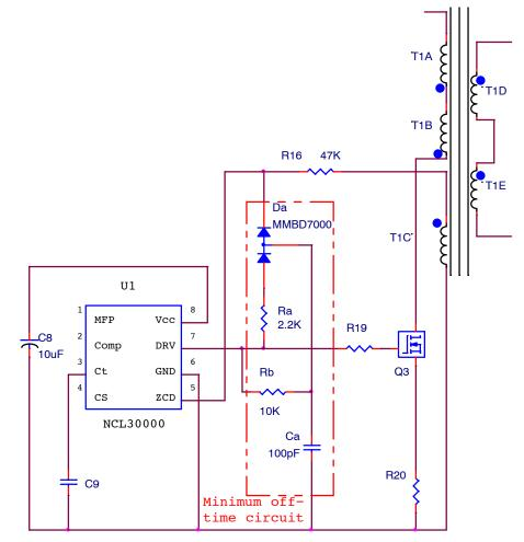
Figure 3. Minimum Off-Time Circuit
