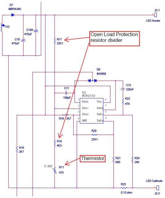
Figure 11. Thermal Foldback Configuration
