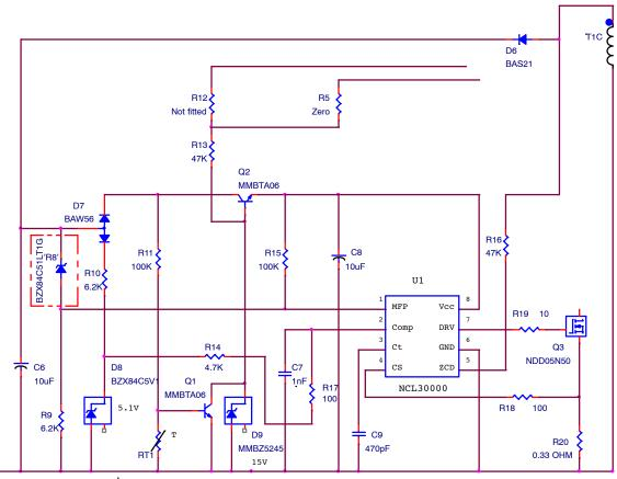
Figure 5. Primary Side Circuitry with OVP and Thermal Shutdown
