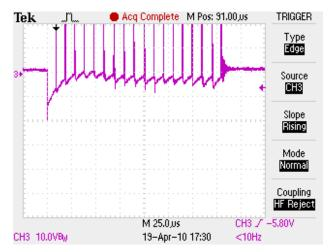
of a high leakage inductance transformer under short circuit. Note the higher switching frequency.
